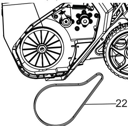
5. Using a socket wrench, remove the large pulley (23).
