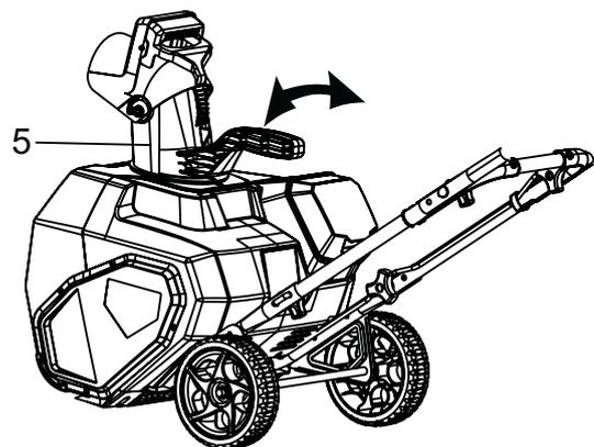
You can adjust the discharge chute 180° to change the snow direction.
