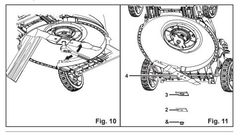
NOTE: Be sure to replace the parts in the exact order in which they were removed. When installing the cutting blade, verify that it is installed with the curved ends pointing toward the mower deck, and not toward the ground. Refer to the schematic drawing on page 28 of this manual.
