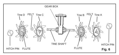
To install the tines, lean the unit back on its wheels so that the handlebar rests on the ground. NOTE: This view of the gearbox for tine installation is from the front of the cultivator.
