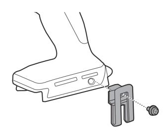
Hand tighten screw with a No. 2 philips head screwdriver.
