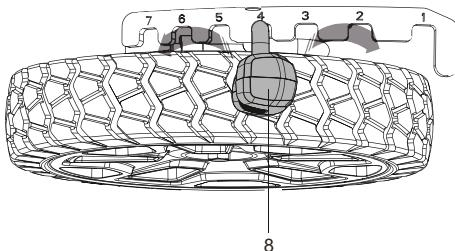
1. Pull the height adjustment lever (8) rearward to increase the blade height.
