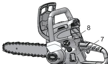
2. Put the oil into the oil tank.
