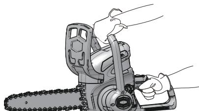
1. Hold the chainsaw with your right hand on the rear handle and left hand on the front handle.
