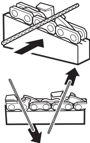
3. Sharpen the top plate, side plate and depth gauge with a flat file.
