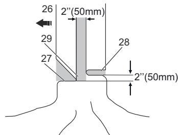
**1. Make a lower-level notching cut (27). Make sure that this cut is:**
