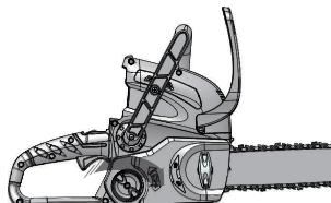
5. When the chain is at the wanted tension, tighten the chain cover.
