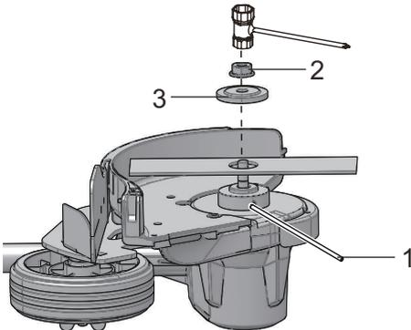
4. Remove the old blade and replace it with a new one.
