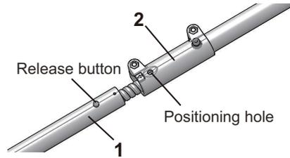
4. Turn the lower shaft until the button locks into the positioning hole.
