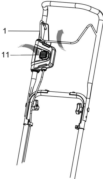
1. While holding the safety switch button (11), pull the bail lever (1) to start the machine.
