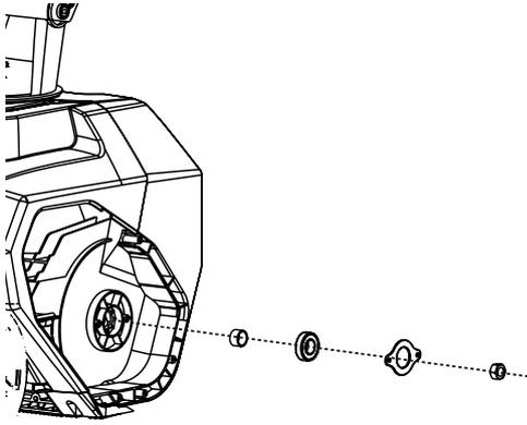
10. Reinstall the left side plate (26), large pulley (23), belt (22) and left side cover (25).
