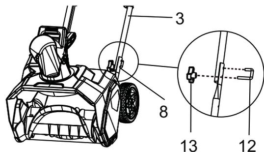
1. Align the holes in the middle handle (3) and the lower handle (8).
