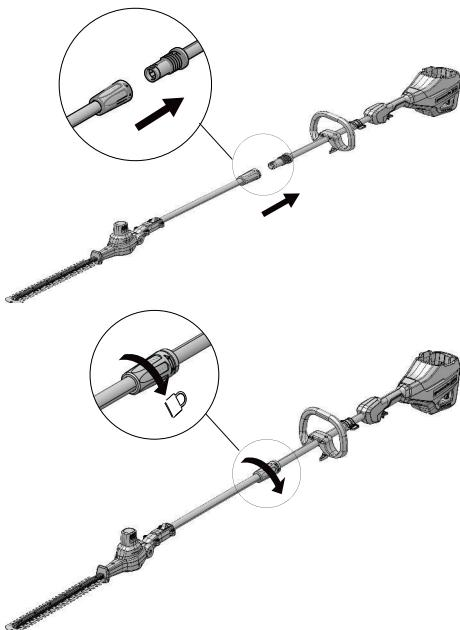
1. Align the handle shaft with the trimmer head.
