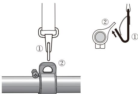
1. Attach the carabiner to the carrying ring on the drive tube.
