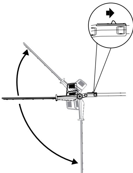
The trimmer head can be locked into 7 positions.
