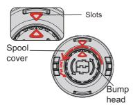
3. Put the cutting line through the hole. Push the cutting line until it exits the opposite hole.
