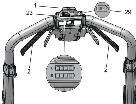
1. Make sure safety key is inserted into slot.
