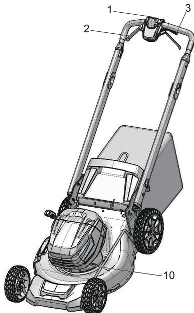
1. When the mower is ready to start, you may grab the start handle (2) or the self-propel lever (3) to turn on the LED headlight (10).
