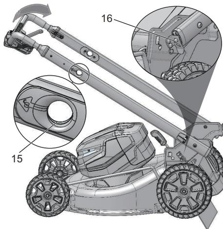
1. Pull up on the handle holes (15) to release the lower handles.
