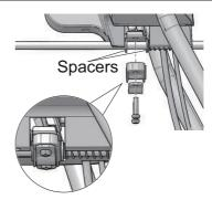
Pull the cable to attach onto bottom of the rod. Align the holes, insert the bolt through the holes and lock with the pin.
