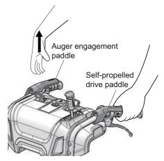
When you push the self-propelled drive paddle (1) and the auger engagement paddle (3) at the same time, the auger engagement paddle will be temporarily locked.
