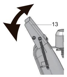
You can adjust the chute deflector up and down to change the throwing distance of the snow.
