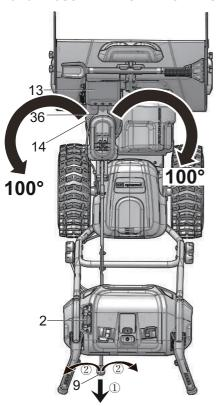
You can adjust the discharge chute  $200^{\circ}$  to change the snow direction.
