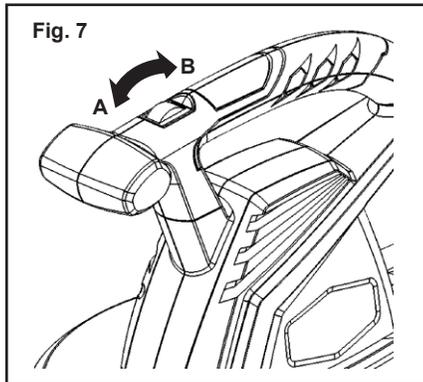
**IMPORTANT:** While in mulching mode the blower **MUST** be in high speed position.
